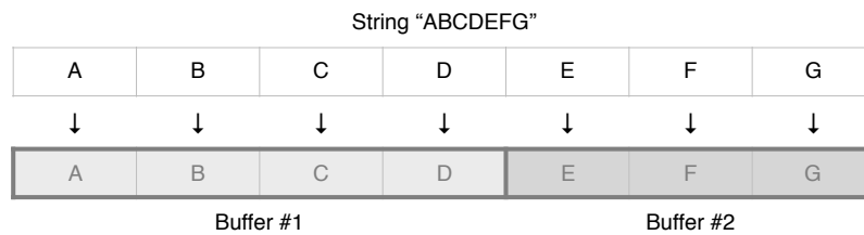
Figure 3.2: Illustration of a buffer overflow: The string "ABCDEFGG" is being copied into Buffer #1, which has insufficient capacity, overflowing and overwriting data in Buffer #2.
